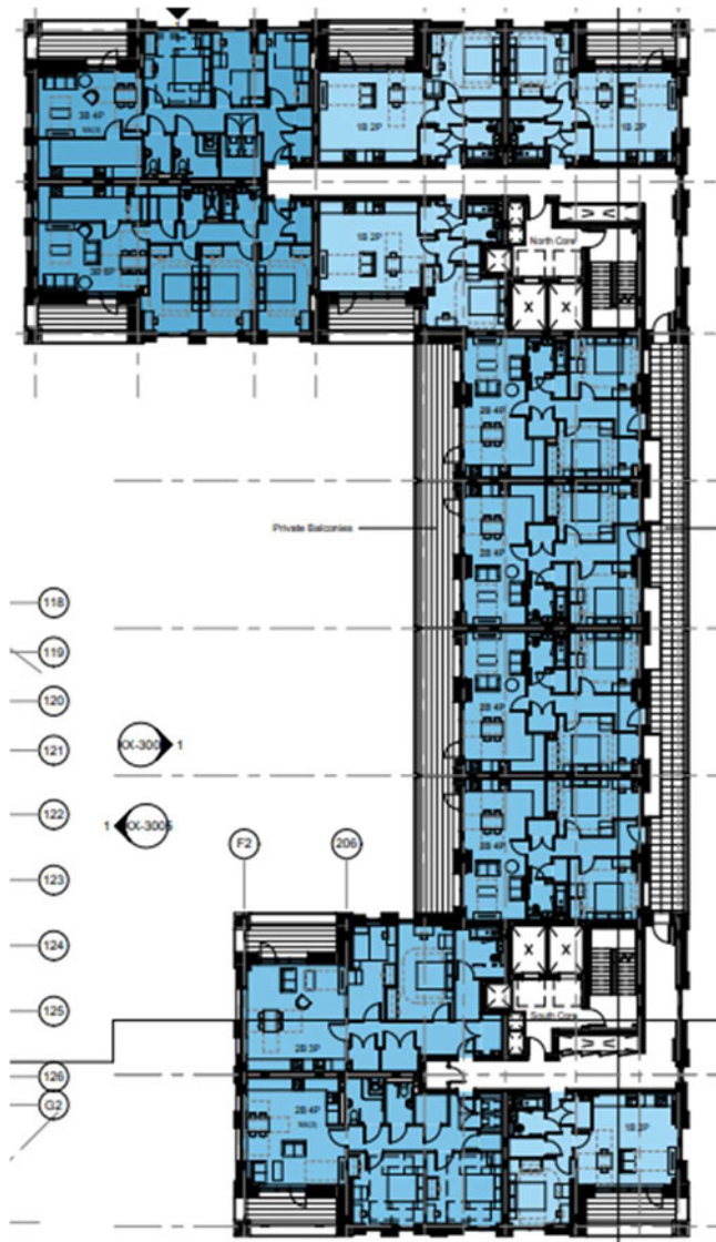
Image above: Typical floorplan for B2 residential block – ground floor duplex units, deck access for central units and north/south core for book end units
